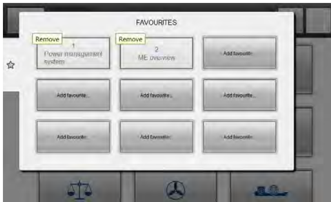
Figure 66 TCP layout – Removing assigned views
