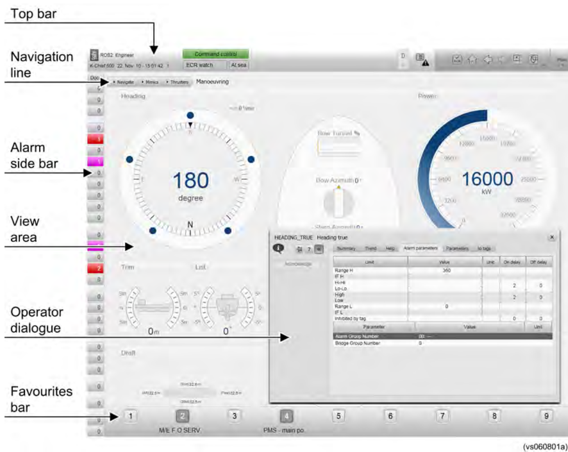
Figure 6 K-Chief 600 main sections
